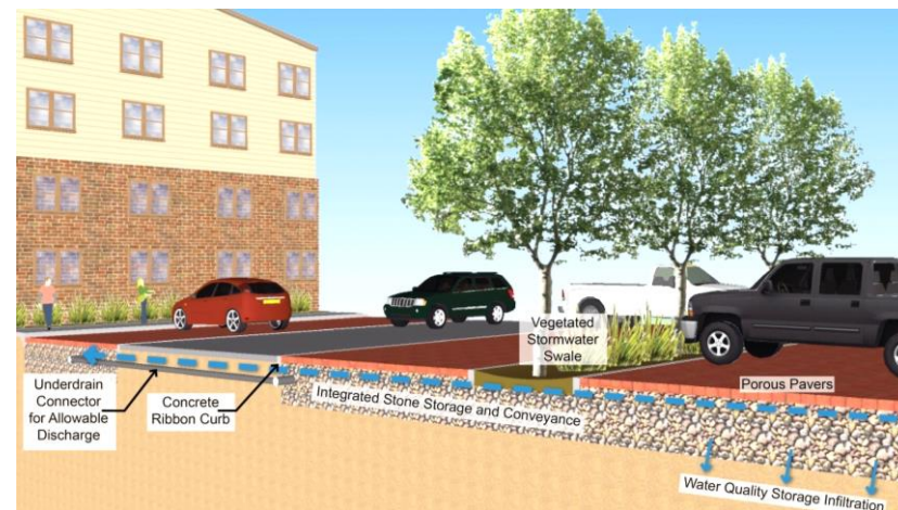
Permeable Paver Parking & Storage Not to Scale
