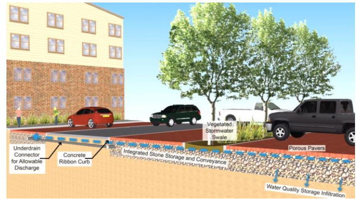
Permeable Paver Parking & Storage Not to Scale
