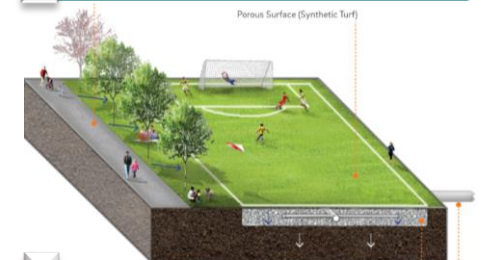
2 Subsurface storage for irrigation reuse
