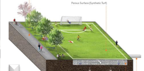
2 Subsurface stormwater management integrated into multi-purpose field (illustrated here).
