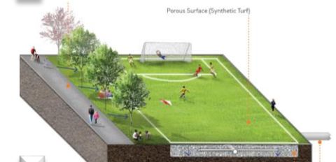
2 Subsurface stormwater management integrated into site amenity
