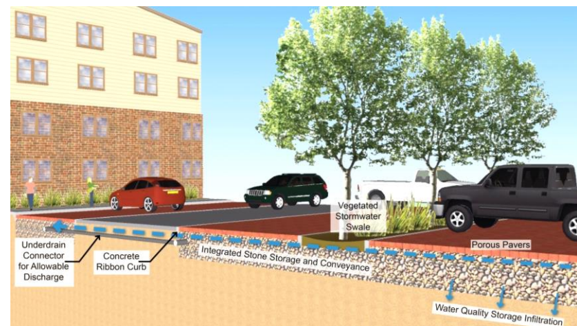
Permeable Paver Parking & Storage Not to Scale
